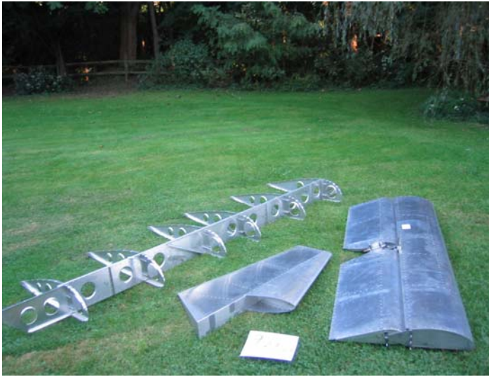
Bob Tedesco with his horizontal tail , rudder and wing skeleton.
