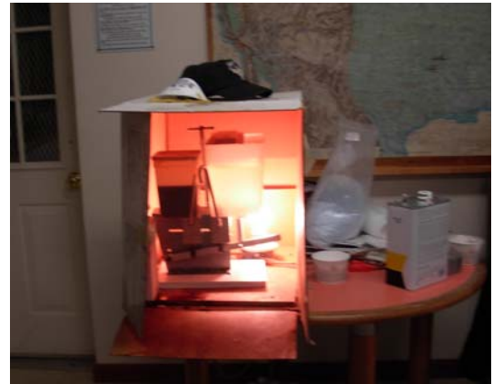
The chemicals must be kept at a controlled temperature. The Kis procedure is to use a cardboard box and a light bulb.
